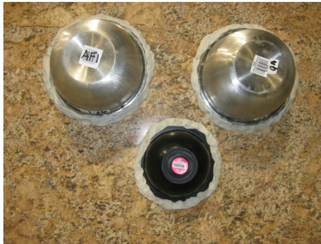
Fig 2 Two discrete component flux monitors and one RFM deployed on a vertical granite surface.
