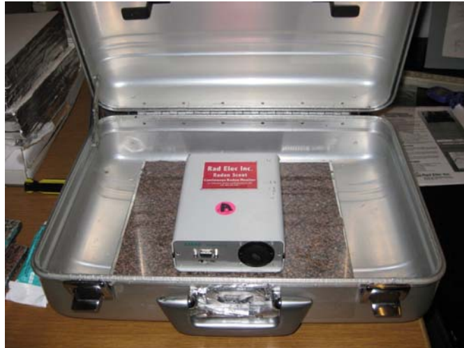
Fig 5 Enclosure accumulator with CRM and granite sample
