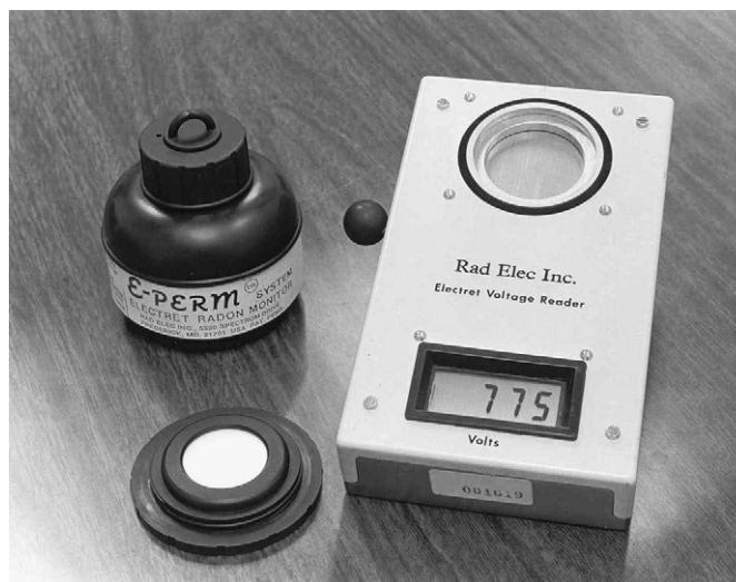
Fig. 1. Electret ion chamber system, chamber, electret (cover removed) and electret reader.
