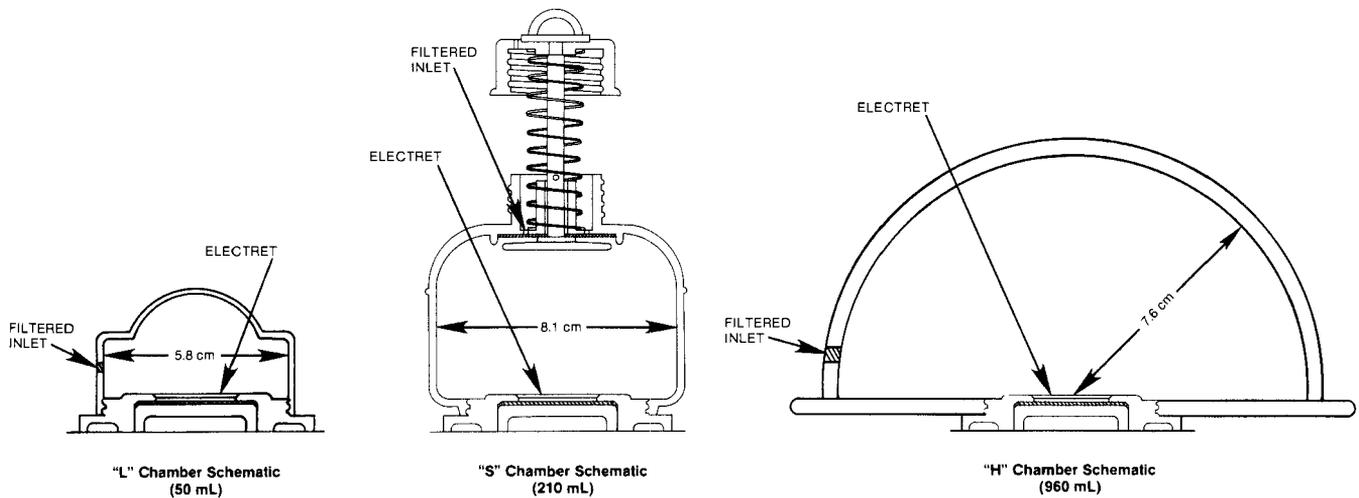
Fig. 1. Schematic of different E-PERM<sup>®</sup> chambers under investigation.
