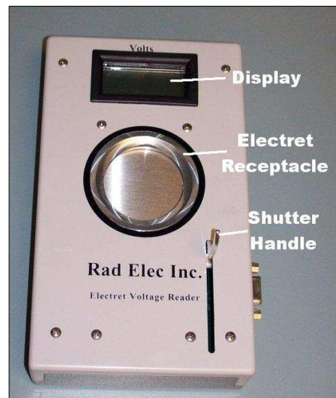
Figure 1 SPER-1E Front Panel
