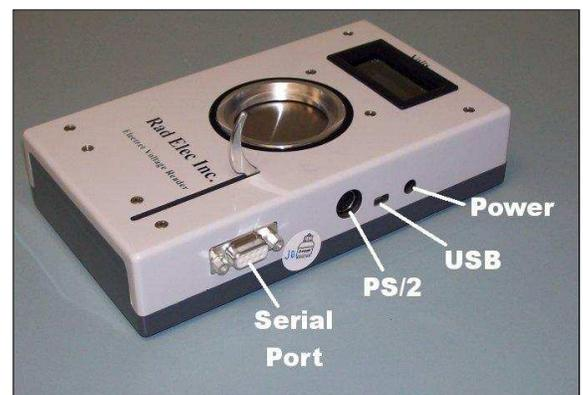
Figure 2 External Connections
