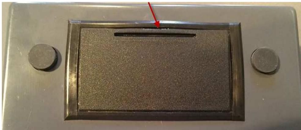
Insert a small flathead screwdriver into the **small slit** and gently push toward the larger slit and lift the lid up. Remove the old batteries. Follow the diagram inside the battery case when inserting the new batteries.
