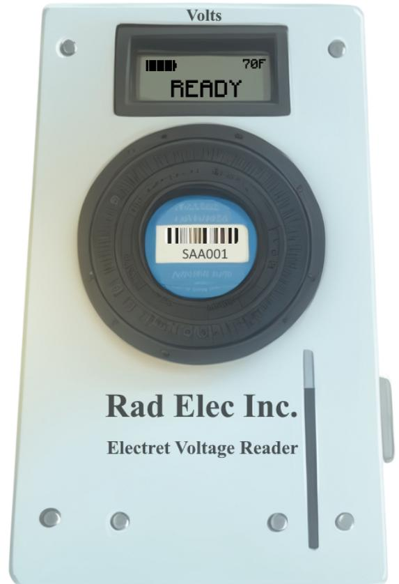
**2** Rotate the electret so that the serial number is parallel (and aligned) with the "Electret Voltage Reader" label etched onto the SPER-1E. For consistency, Rad Elec recommends keeping the reader in its case. Prop it up against the foam inside the case so that it sits at about a 10° angle. This ensures that gravity will pull the electret ever-so-slightly towards you, to remain consistent.
