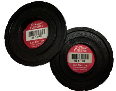
**Reference electrets are never to be used for radon testing.**
