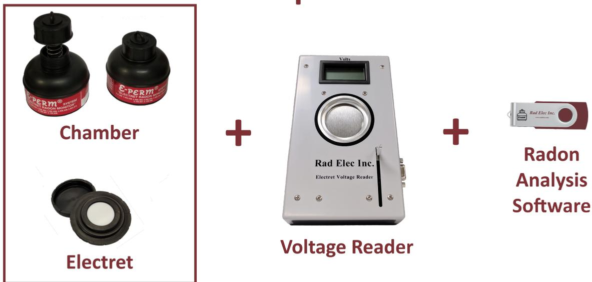
These components are needed to make both short-term and long-term radon measurements, and can be used either indoors or outdoors. When an electret is loaded onto an ion chamber it is called an E-PERM®, which is also referred to as an electret ion chamber (EIC).
