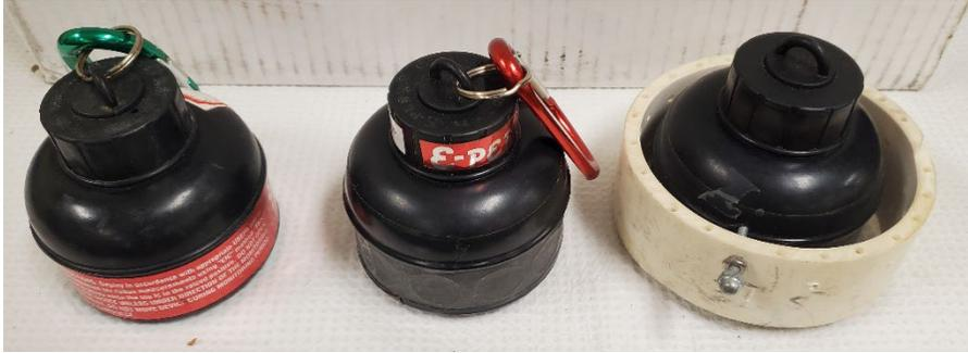
Figure (1): E-PERM chambers used, left to right: S, RT, modified-RT.
