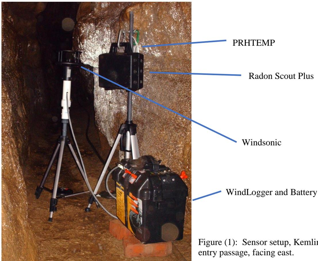
Figure (1): Sensor setup, Kemling Cave entry passage, facing east.
