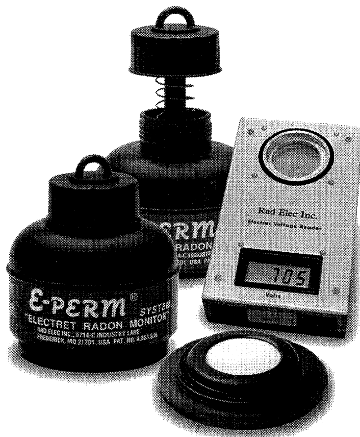
Figure 1. Components of electret ion chambers. Electret, chamber and reader.
