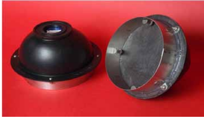
FIG. 2. Radon Flux monitors with aluminium collars for in-soil installation [7].
